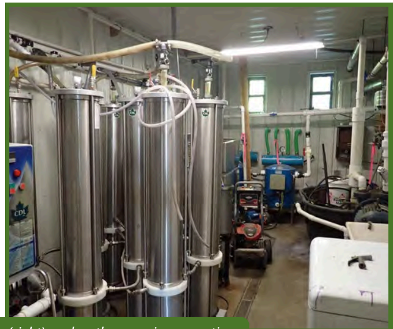
The 5'x15' CDL oil-fired evaporator (left) and 8-post RO system (right) anchor the sugaring operation.
