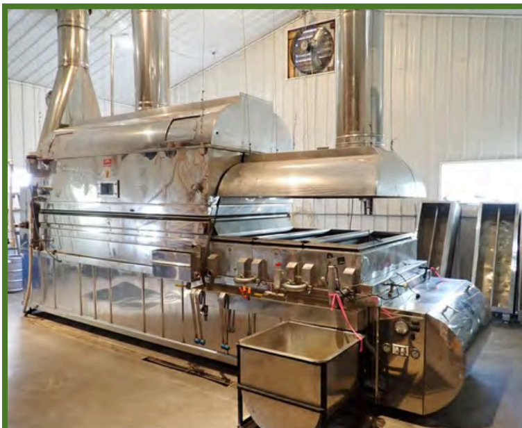
The 5'x15' CDL oil-fired evaporator (left) and 8-post RO system (right) anchor the sugaring operation.
